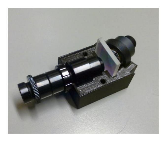
Researchers used 3-D printing to make the holder (black rectangular piece) for the optics used to create an inexpensive and small hyperspectral imager. Feasibility tests showed that 3-D printing can be used to produce prototype parts that are accurate enough for optical systems. Credit: Fred Sigernes, University
