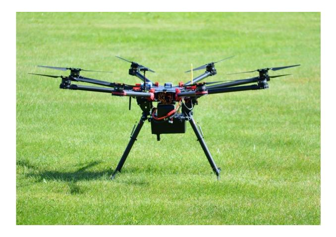
Researchers used 3-D printing to create hyperspectral imagers that are light enough to use on a drone. The imager is the small protrusion on the bottom of
