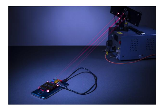
The wireless charging system created by University of Washington engineers. The charging laser and guard lasers are normally invisible to the human eye, but red beams have been inserted in place of the guard beams for demonstration purposes. Credit: Mark Stone/University of Washington
