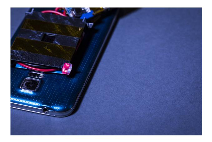
Illuminated in red is one of the 3-D printed retroreflectors, which reflects the low-power guard beams to diodes on the laser emitter. Interruption of the guard beams triggers a safety system which blocks the charging beam. Credit: Mark Stone/University of Washington
