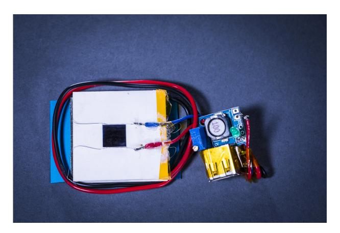
The UW team's prototype heatsink assembly, which can be attached to the back of a smartphone, consists of a photovoltaic cell (silver square, top) attached to a thermoelectric generator (in white). The generator is mounted on top of an aluminum heatsink. The entire assembly is only 8mm thick and 40mm wide. Credit: Mark Stone/University of Washington
