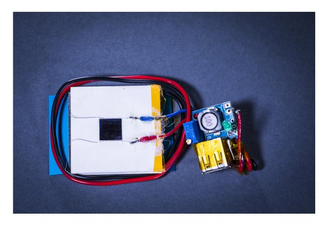
The UW team's prototype heatsink assembly, which can be attached to the back of a smartphone, consists of a photovoltaic cell (silver square, top) attached to a thermoelectric generator (in white). The generator is mounted on top of an aluminum heatsink. The entire assembly is only 8mm thick and 40mm wide. Credit: Mark Stone/University of Washington
