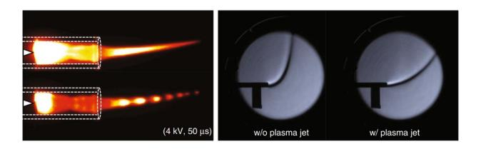
(Top left) Image of the plasma jet in continuous mode and (bottom left) composite image of nanosecond-resolved images. (Right) Schlieren photography images of the trajectory of gas flow with and without a plasma jet. Credit: Park et al. Published in *Nature Communications*
