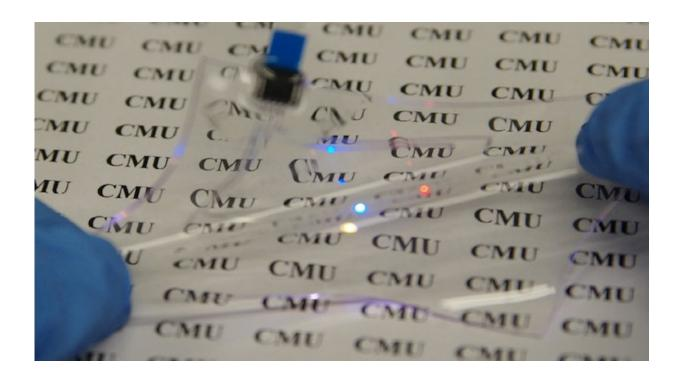
The displays and touchscreens used in next-generation technologies will require transparent conductors that are soft, elastic, and highly stretchable. Credit: Soft Materials Laboratory, Carnegie Mellon University
