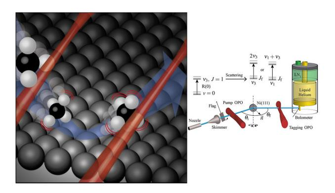
Illustration of methane scattering from a Ni(111) surface (left) and a diagram of the experimental setup used in this study (right). Credit: Rainer Beck/EPFL
