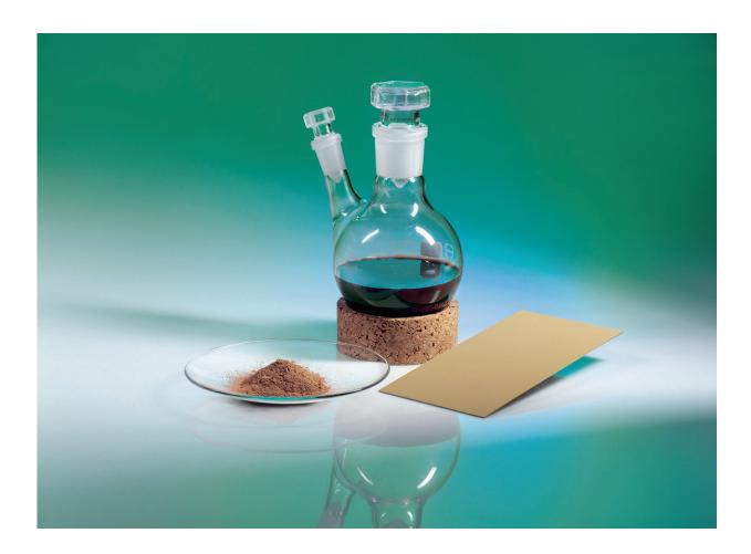
Lignin is a real alternative to fossil resources in the manufacture of primers and adhesives. Credit: Fraunhofer IFAM
