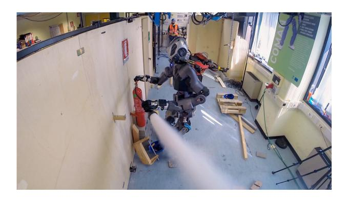
the WALK-MAN humanoid robot is thought for supporting emergency response teams. The robot is also able to activate an extinguisher to eliminate the fire. Credit: IIT-Istituto Italiano di Tecnologia
