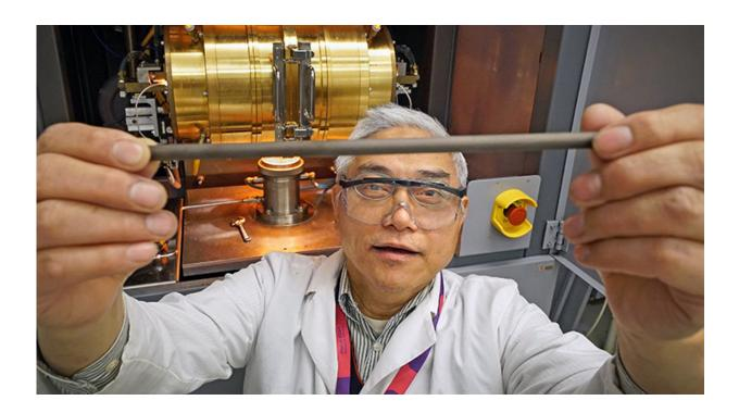
Physicist Genda Gu holds a single-crystal rod of LBCO—a compound made of lanthanum, barium, copper, and oxygen—in Brookhaven's state-of-the-art crystal growth lab. The infrared image furnace he used to synthesize these high-quality crystals is pictured in the background. Credit: Brookhaven National Laboratory
