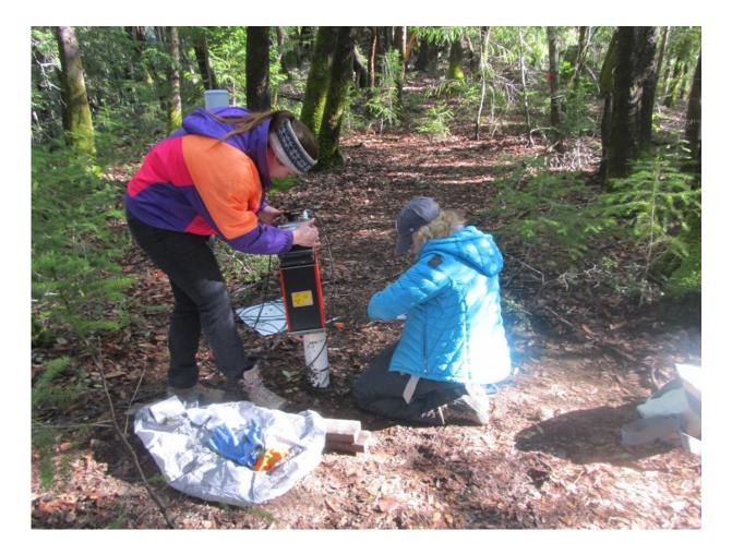
Researchers at the field site using a neutron probe to measure rock moisture inside of a borehole. Credit: The University of Texas at Austin Jackson School of Geosciences.
