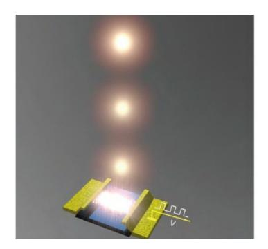
Researchers have demonstrated graphene-based devices that emit ultrafast light pulses with a duration of less than 100 picoseconds (1 picosecond = 1 trillionth of a second). Credit: Kim et al. ©2018 American Chemical Society
