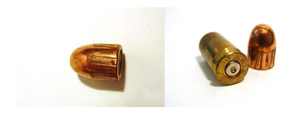
A fired bullet with rifling impressions from the barrel of a gun (left). A fired cartridge case and fired bullet (right). Experts can often identify the weapon used based on rifling impressions on the bullet or impressions on the primer (the silver-colored metal) at the base of the cartridge case. Credit: Robert Thompson/NIST
