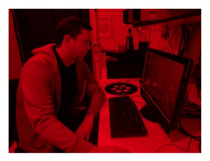
Luminescence dating samples being measured under controlled lighting conditions at the University of Adelaide's Prescott Environmental Luminescence Laboratory. Credit: Lee Arnold
