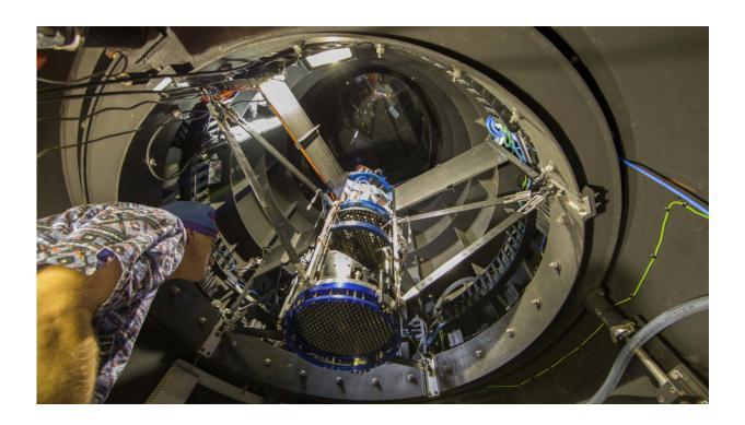
The TAIPAN facility on the UK Schmidt Telescope will use a new technology involving mini robots known as Starbugs. Credit: Australian National University
