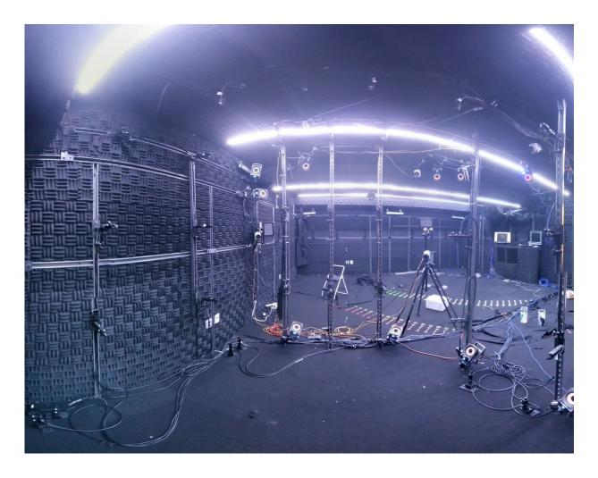
A panoramic view of the "bat lab" at Johns Hopkins University taken during experiment preparation shows the multiple cameras and ultrasonic microphones used to capture a bat's sonar signal during flight. During the actual sonar experiments the cables were tidied up and all exposed metal surfaces were covered by felt. Credit: Benjamin Falk/Johns Hopkins University
