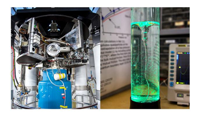
Rotating cryostat with the superfluid helium near absolute zero (left); a novelty model of a vortex inside a container (right) similar to the one inside the cryostat. The actual vortices are perfectly even, whereas in the model, the vortex varies in thickness. Credit: Aalto University
