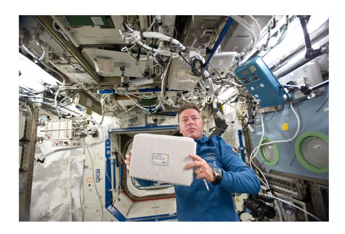
ESA astronaut Roberto Vittori on the International Space Station in 2011 with the air quality control and monitoring system NADIR developed to check for possible anomalies in the internal atmosphere on the station. NADIR was part of the IENOSE Experiment. Credit: NASA
