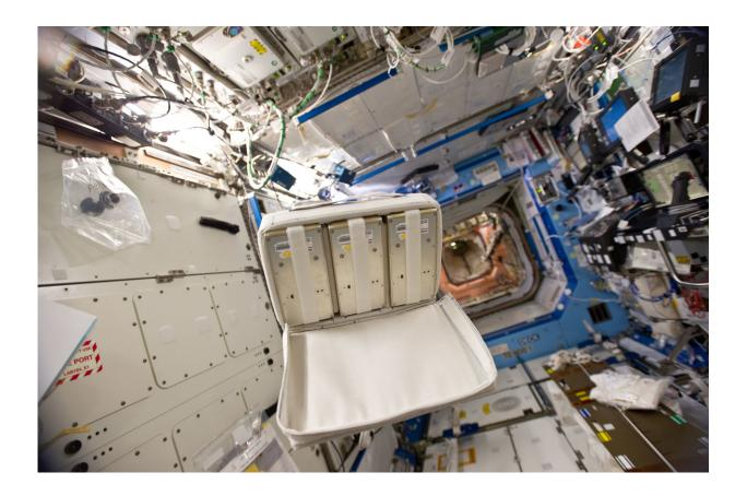
The air quality control and monitoring NADIR system, part of the IENOSE Experiment, were installed on the International Space Station in 2011 by ESA astronaut Roberto Vittori. It consisted of 3 sensor units to be positioned in different locations on the station. Credit: NASA
