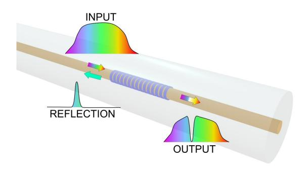
Fiber Bragg gratings are used to turn an optical fiber into a sensing element by reflecting a specific wavelength back in the direction from which it came. New dissolvable fiber Bragg gratings can be used as sensors in the body and are safe even if the fiber were to accidently break inside the patient. Credit: Maria Konstantaki, Foundation of Research and Technology - Hellas
