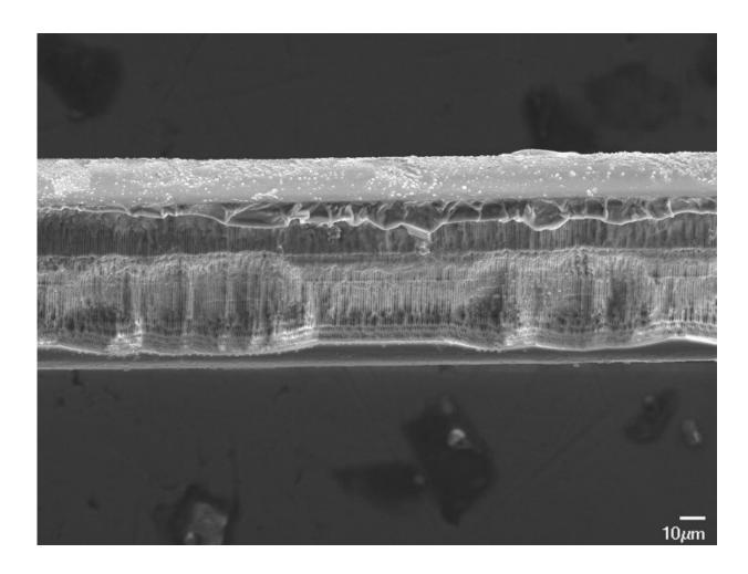
Researchers inscribed a sensing element known as fiber Bragg grating into a glass optical fiber designed to dissolve completely inside the body. The image
