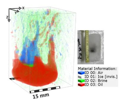
Here's what the visualization technology shows researchers, with a puddle of oil at the bottom of the sample and brine and a big pocket of air. In spite of these obstructions in the ice, the oil has still been able to migrate upwards in the ice towards the surface. Credit: Martina Lan Salomon, NTNU
