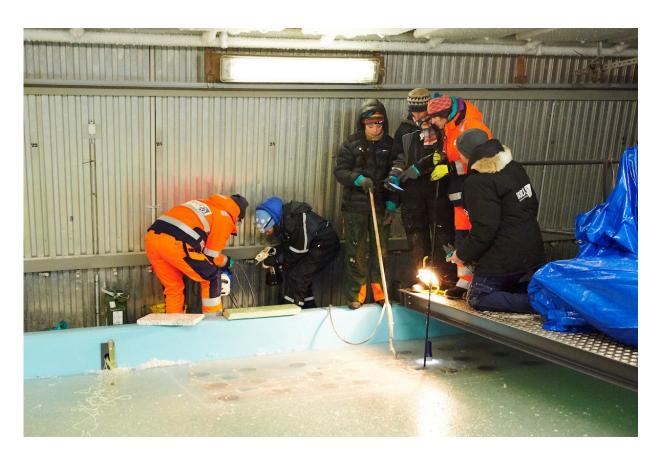
Researchers inject oil into the different ice samples. The 32 samples are all injected with oil at the same time, and then researchers can take samples each day from a different core to see how the oil moves over time. Credit: Giuliani von Giese, Hamburg
