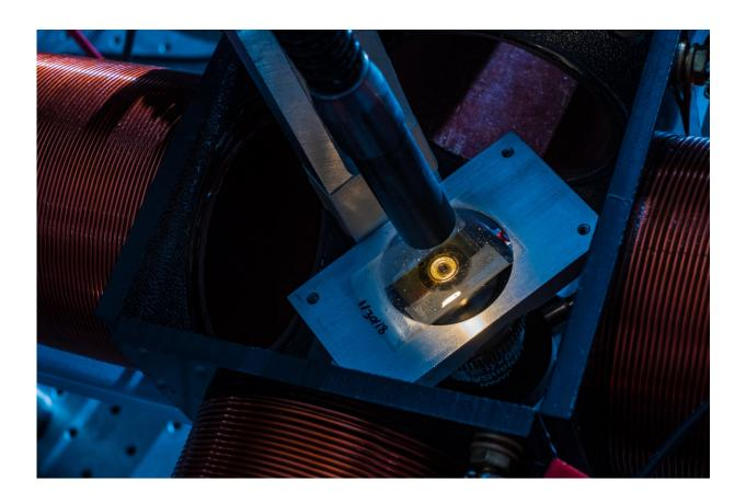
Micron-sized magnetic particles are set to go for a spin in a custom rig used by Rice University to study the effects of a spinning magnetic field on materials. Credit: Jeff Fitlow/Rice University
