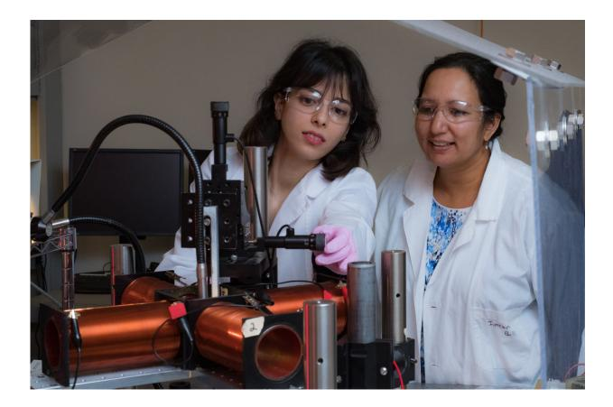
Rice University graduate student Elaa Hilou (left) and Professor Sibani Lisa Biswal set up an experiment in a device that combines a rotating magnetic field and a microscope. The researchers are studying the effects of a spinning field on
