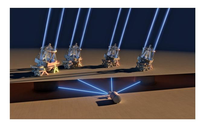
The ESPRESSO instrument on ESO's Very Large Telescope in Chile has used the combined light of all four of the 8.2-meter Unit Telescopes for the first time. Combining light from the Unit Telescopes in this way makes the VLT the largest optical telescope in existence in terms of collecting area. This picture shows in highly simplified form how the light collected by all four VLT Unit Telescopes is combined in the ESPRESSO instrument, located under the VLT platform. Credit: ESO/L. Calçada
