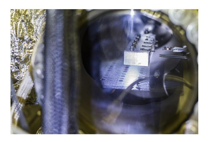
Extreme conditions are used to protect and preserve the TMDs during the experiments. As shown here, all samples are stored and manipulated in a vacuum that is close to the conditions in space. Credit: Kyle Mittan
