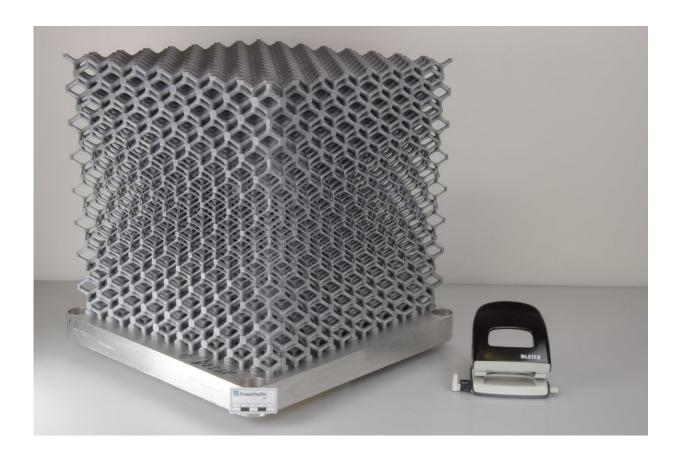
Lattice cube with edge length of 40 centimeters, one of the largest metal structures manufactured using selective laser melting (SLM). Credit: Fraunhofer EMI
