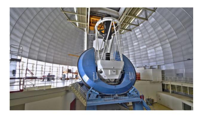
A view inside the dome at the Mayall Telescope near Tucson, Arizona. The 2-meter corrector barrel atop the telescope will be removed and replaced with a new corrector barrel for the Dark Energy Spectroscopic Instrument. DESI's installation will begin soon. Credit: P. Marenfeld and NOAO/AURA/NSF
