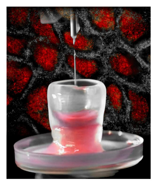
A tube with an outer diameter of approximately 15 mm and a modular internal architecture is printed in one step, by depositing core-shell alginate microparticles onto a rotating substrate. The nozzles are just visible in the top of the image. Credit: C.W. Visser and T. Kamperman
