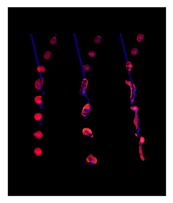
In-air impact of jets (in blue, flowing from the top-left) onto a train of droplets (in red, flowing from the top-right). After impact, the droplets are coated by the jet's liquid, as the jet's surface tension is lower. By adding a solidifying agent to the jet, the droplets can be solidified into particles in milliseconds, and collected
