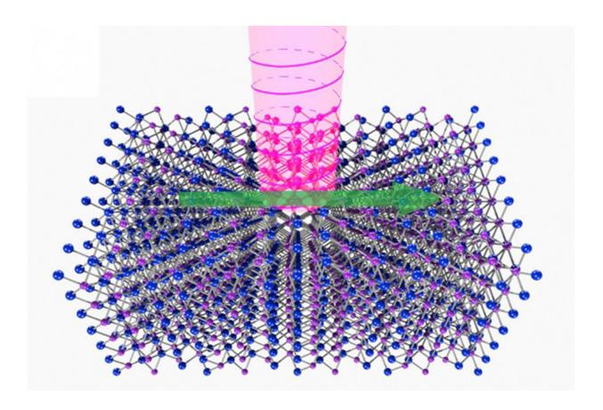
Scientists predicted and directly measured electrons in a semimetal. The electrons were behaving like elusive massless particles. Shining a circularly polarized light beam (pink spiral) onto a tantalum-arsenide semimetal (ball-and-stick crystal model) generates an electrical current (green arrow). Remarkably, the direction of the current flow changes by switching the light's polarization from right-handed to left-handed, proving the handedness of exotic Weyl
