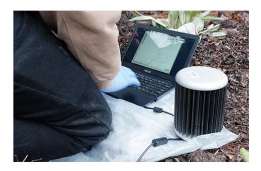
This simple on-site equipment uses a polymerase chain reaction technique to let farmers do cheap, fast and accurate on-site soil testing for crop-damaging pathogens. Credit: Washington State University
