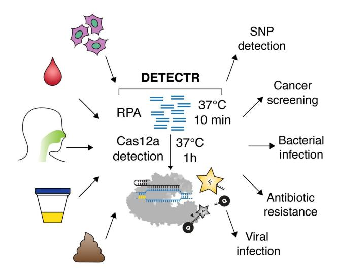
The new DETECTR system, created at UC Berkeley based on CRISPR-Cas12a, can analyze cells, blood, saliva, urine and stool to detect genetic mutations, cancer and antibiotic resistance as well as diagnose bacterial and viral infections. It works by amplifying target DNA with the RPA system, and using a fluorescent reporter (F star) tied to single-stranded DNA to signal Cas12a has found its target. Credit: Doudna lab, UC Berkeley
