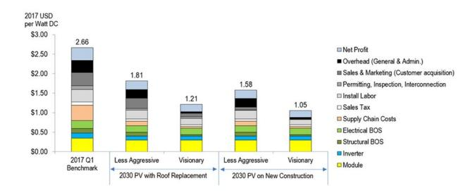
Modeled installed system costs of PV at time of roof replacement and new construction as compared to NREL's 2017 Q1 benchmark. Credit: National Renewable Energy Laboratory
