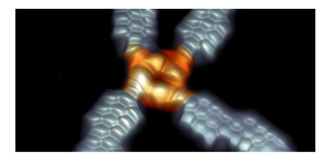
Scanning Tunneling Microscopy image of the new molecular device and its graphene nanoribbons contacts. Credit: CIC nanoGUNE
