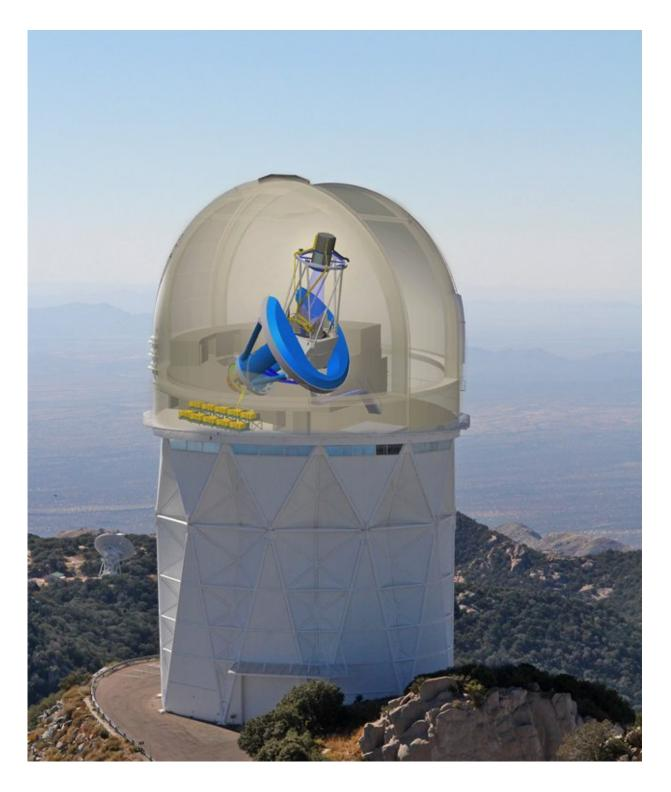
The Dark Energy Spectroscopic Instrument (DESI) will be mounted on the Kitt Peak Mayall telescope. Light from galaxies and quasars will be collected at prime focus by robotically positioned fibers and fed to 10 spectrographs. Credit: R. Lafever, J. Moustakas/DESI Collaboration, P. Marenfeld/NOAO/AURA/NSF
