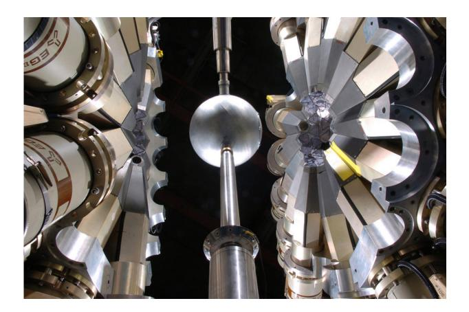
Argonne scientists and collaborators used the Gammasphere, this powerful gamma ray spectrometer, to help create the right conditions to cause and spot a long-theorized effect called nuclear excitation by electron capture. Credit: Argonne National Laboratory
