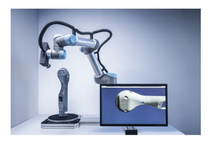
The scanning system is able to measure any component in real time, making protracted teaching processes a thing of the past. Credit: Fraunhofer IGD
