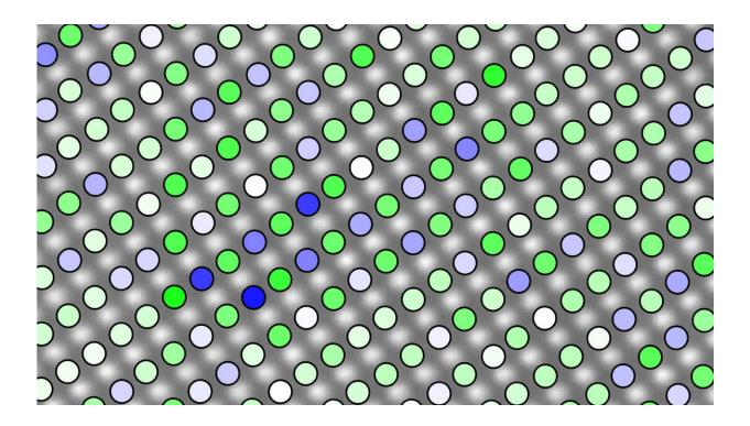
Atomic resolution image illustrating the chemical distribution in lead magnesium niobate. Due to mass contrast, columns of atoms rich in magnesium (blue markers) can be discriminated from columns rich in niobium (green markers). Credit: James LeBeau
