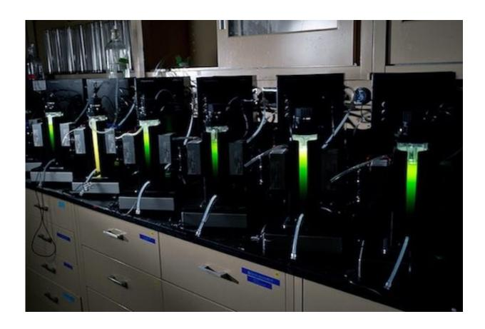
Algae were stress tested in these bioreactors made in the Kramer lab. Each is a 'pond in a jar' that can reproduce real-world settings for testing purposes. Credit: G.L. Kohuth
