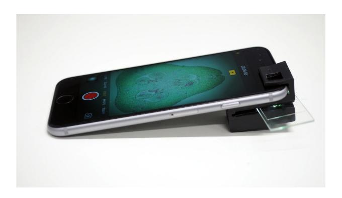
Add-on clip turns smartphone into fully operational microscope. Credit: CNBP
