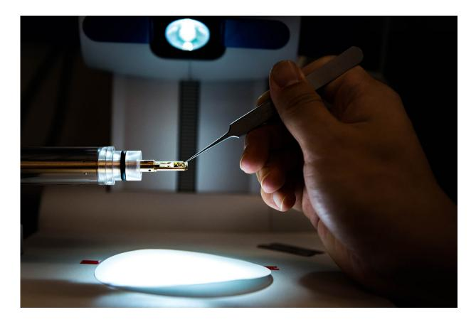
A sample is readied for analysis using a transmission electron microscope. Credit: Purdue University image/Marshall Farthing
