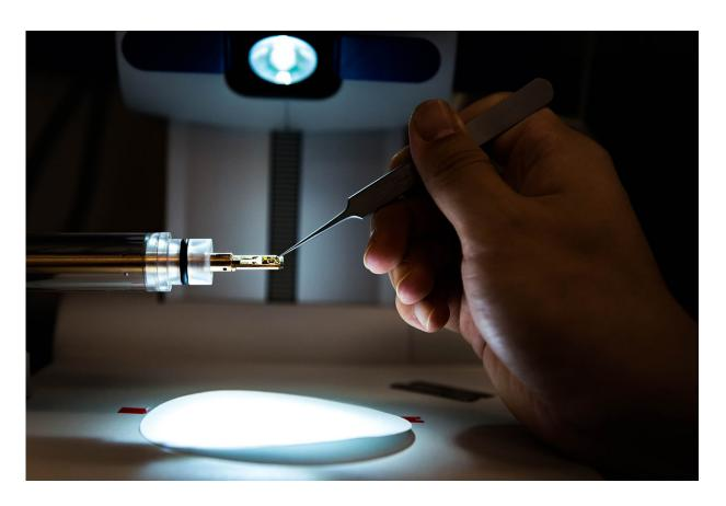
A sample is readied for analysis using a transmission electron microscope. Credit: Purdue University image/Marshall Farthing
