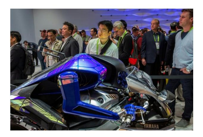
Yamaha's 'Motoroid' concept electric motorcycle reaches speeds topping 200 kilometers per hour but is blind, relying on pre-programmed routes
