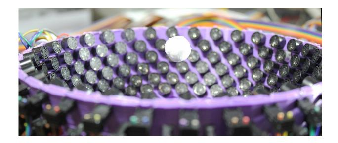
A styrofoam particle of 1.6cm (1.88 wavelengths of sound) trapped in the centre of a 40kHz ultrasonic generator of virtual vortices. Credit: University of Bristol
