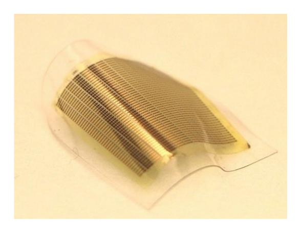
Wavy transistor arrays represent a step toward developing a single gadget with shape and size that can be dynamically reconfigured. Credit: Muhammad M. Hussain
