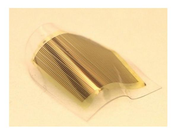
Wavy transistor arrays represent a step toward developing a single gadget with shape and size that can be dynamically reconfigured. Credit: Muhammad M. Hussain
