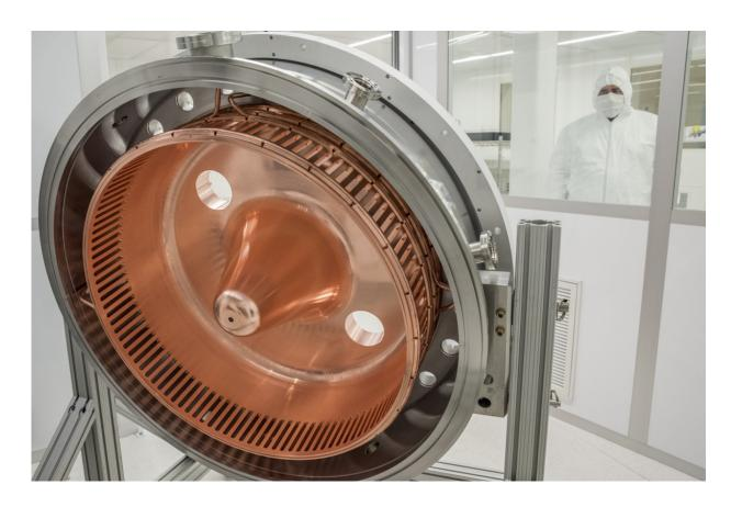
A copper cone structure inside the injector gun's central cavity. Credit: Marilyn Chung/Berkeley Lab
