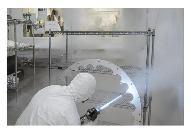
Joe Wallig, a mechanical engineering associate, prepares a metal ring component of the injector gun for installation using a jet of high-purity dry ice in a clean room. Credit: Marilyn Chung/Berkeley Lab
