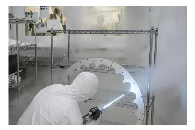
Joe Wallig, a mechanical engineering associate, prepares a metal ring component of the injector gun for installation using a jet of high-purity dry ice in a clean room. Credit: Marilyn Chung/Berkeley Lab
