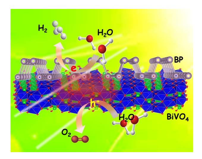
Fig.2. Photocatalytic overall pure-water splitting using the 2D heterostructures of BP/BiVO4 without any sacrificial agents under visible light irradiation. Credit: Osaka University
