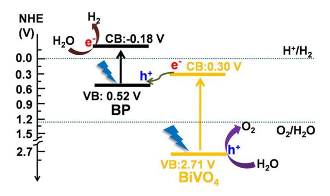
Fig.1. Schematic diagram of Z-scheme photocatalytic overall water splitting using BP/BiVO4 under visible light irradiation. Credit: Osaka University
