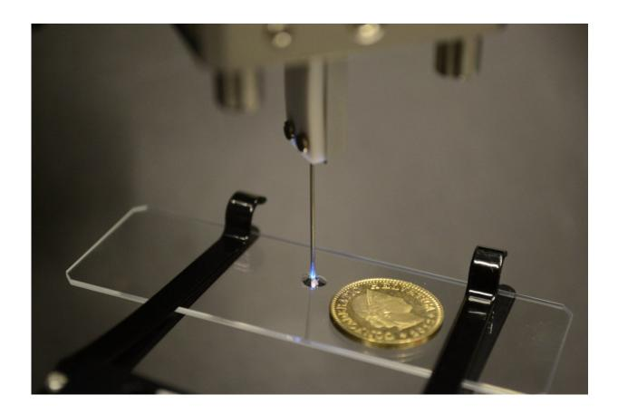
Researchers used an optical fiber housed inside the needle pictured to deliver light for 3-D printing microstructures. The light selectively hardens volumes inside the droplet of photopolymer on the glass slide. The new system could one day allow 3-D printing inside the body. Credit: Damien Loterie and Paul Delrot, École Polytechnique Fédérale de Lausanne
