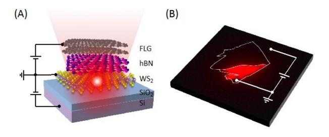
Figure shows the emission of red light from an electrically excited LED fabricated with 2D semiconductor materials. (A) The left image illustrates the device structure consisting of various layered materials. The stack of layers consist of few-layer graphene (FLG), hexagonal boron nitride (hBN) and tungsten disulfide (WS2). (B) The right image shows a microscope image taken in the dark while a voltage is applied to the device. Credit: National University of Singapore
