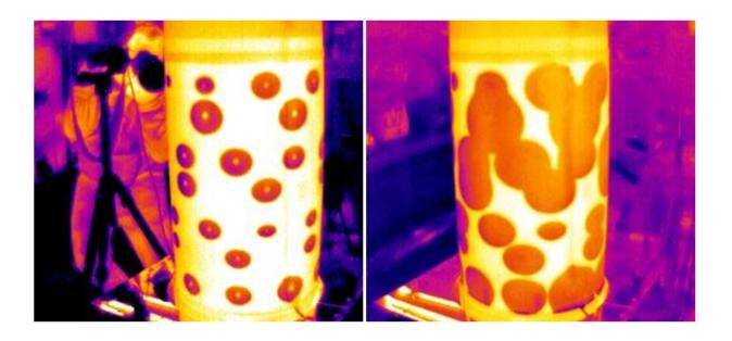
Empa's sweat torso ejects precisely defined quantities of liquid through a large number of small nozzles during the experiments. Credit: Swiss Federal Laboratories for Materials Science and Technology
