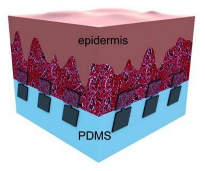
An illustration shows how the "dumbbells," (in grey) hook into the layer of blue
