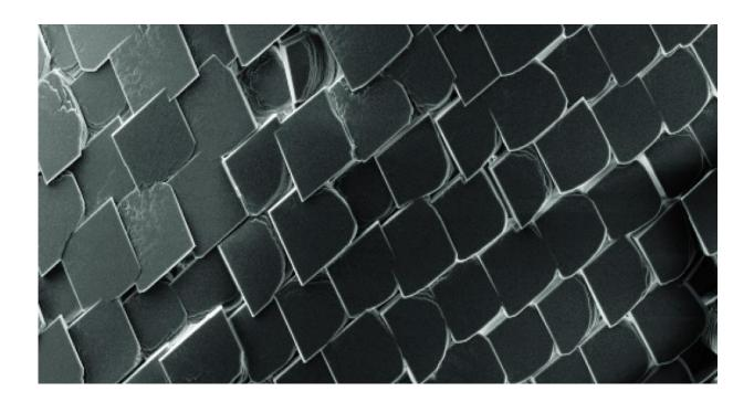
A scanning electron microscope picture shows the artificial "scales," about a dozen of which could fit across the period at the end of a sentence. Credit: Tian lab/University of Chicago
