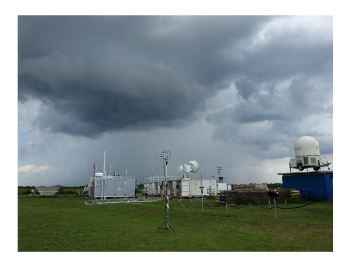
A heavily instrumented ground site downwind of Manaus captured measurements of aerosols, clouds, and solar and thermal energy during GoAmazon. Credit: US Department of Energy ARM Climate Research Facility
