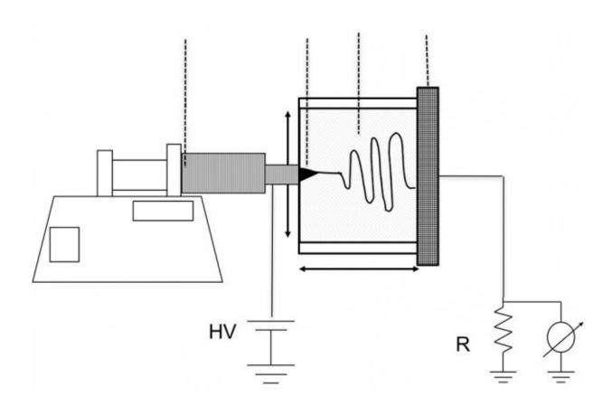
A diagram of the device used to produce the fibers shows a heated syringe (left) through which the solution is extruded, and a chamber (right) where the strands are subjected to an electric field that spins them into the highest performing polyethylene fibers ever made. Credit: Massachusetts Institute of Technology
