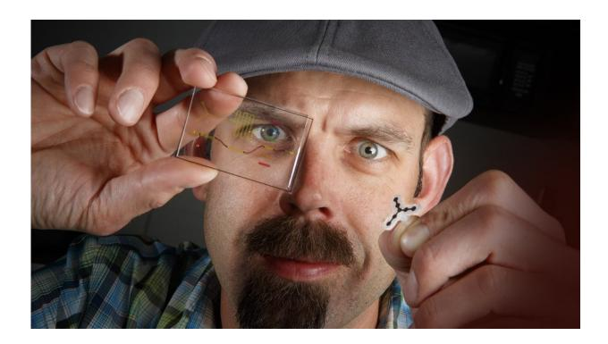
Stephen Morin and his colleagues have detailed a method for more strongly bonding plastics with silicones, offering new possibilities for fabricating fluidcarrying channels (left) that are commonly used to direct the motion of soft robotic components (right). Credit: University of Nebraska-Lincoln
