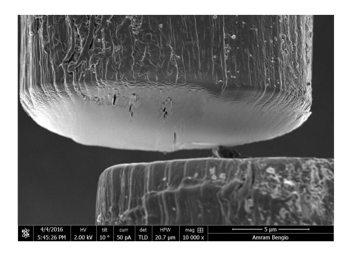
Thread-like fibers created with a new, rapid method at Rice University are made of billions of carbon nanotubes that can be quickly aligned by shear force between slides. Credit: Complex Forms of Complex Fluids/Rice University
