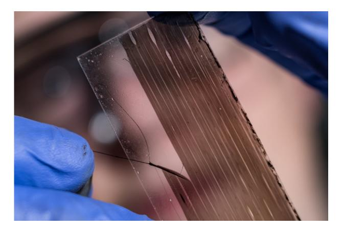
Rice University graduate student Robby Headrick peels a strip of aligned carbon nanotubes from a slide. The lab's method for making short nanotubes takes weeks off the time needed to make samples for testing. Credit: Jeff Fitlow/Rice University
