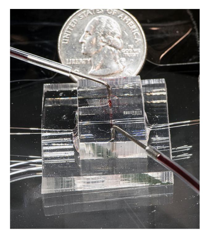
Close-up of a microflow system with red dye in fluid channel. Credit: NIST
